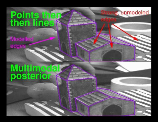
Strong unmodelled edges frequently break the edge tracker
