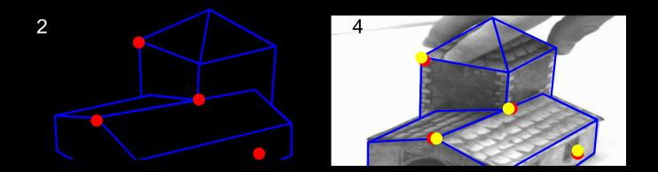
Project features on to model. Drift occurs here Alter pose to minimize reprojection error
