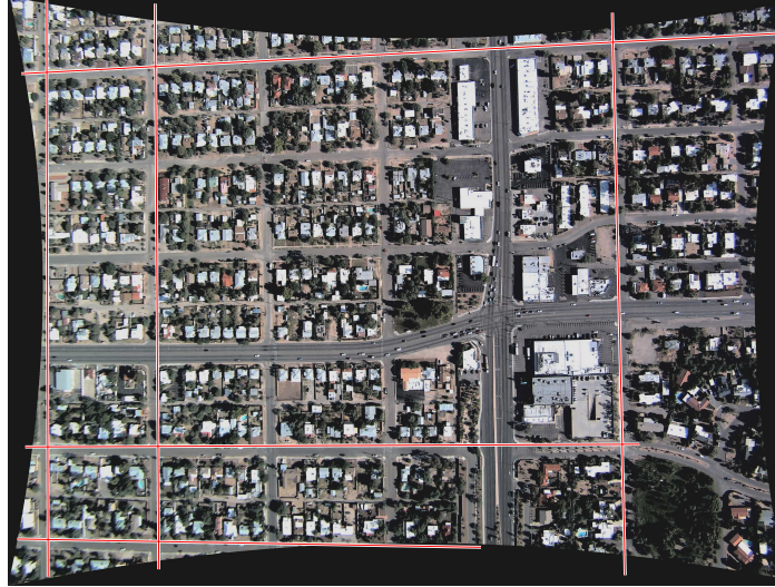
Figure 2. This shows a radially corrected version of a frame; lines have been superimposed to allow comparisons for straightness.
