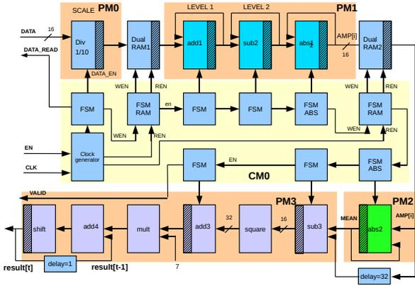
Figure 1: Level-2 Haar wavelet, mean and variance FPGA implementation
