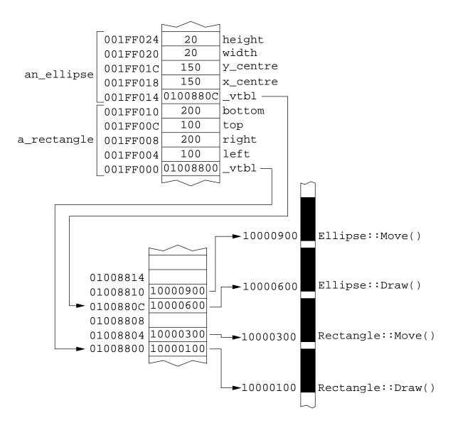
Note that we use a double indirection to avoid duplicating a large set of pointers for every instance of the object.
