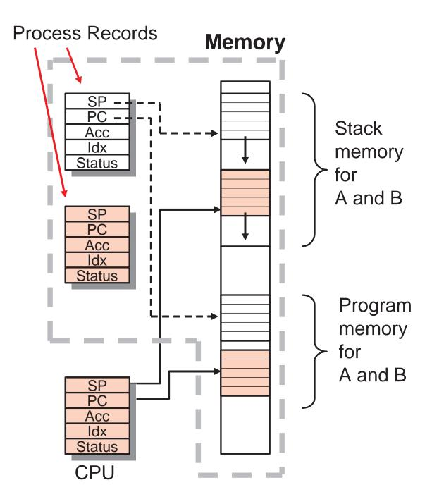
Context Switch: (a) save current cpu reg; (b) load new cpu reg
