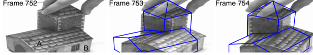
Figure 4: Three consecutive video frames are shown while the model rotated rapidly (about 720^\circ/s ) around its centre. The outline indicates the position of the model in the previous frame. Features on face A change appearance and features on face B change shape significantly.
