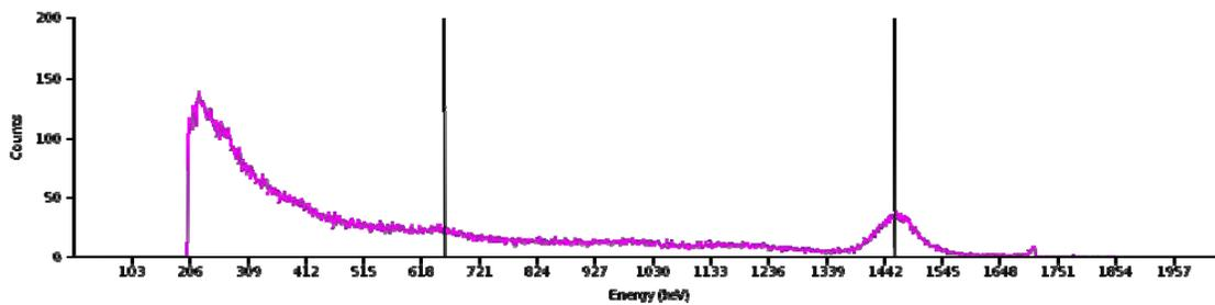
Figure 9 Signal and background spectra for a vehicle without radioactive material.
