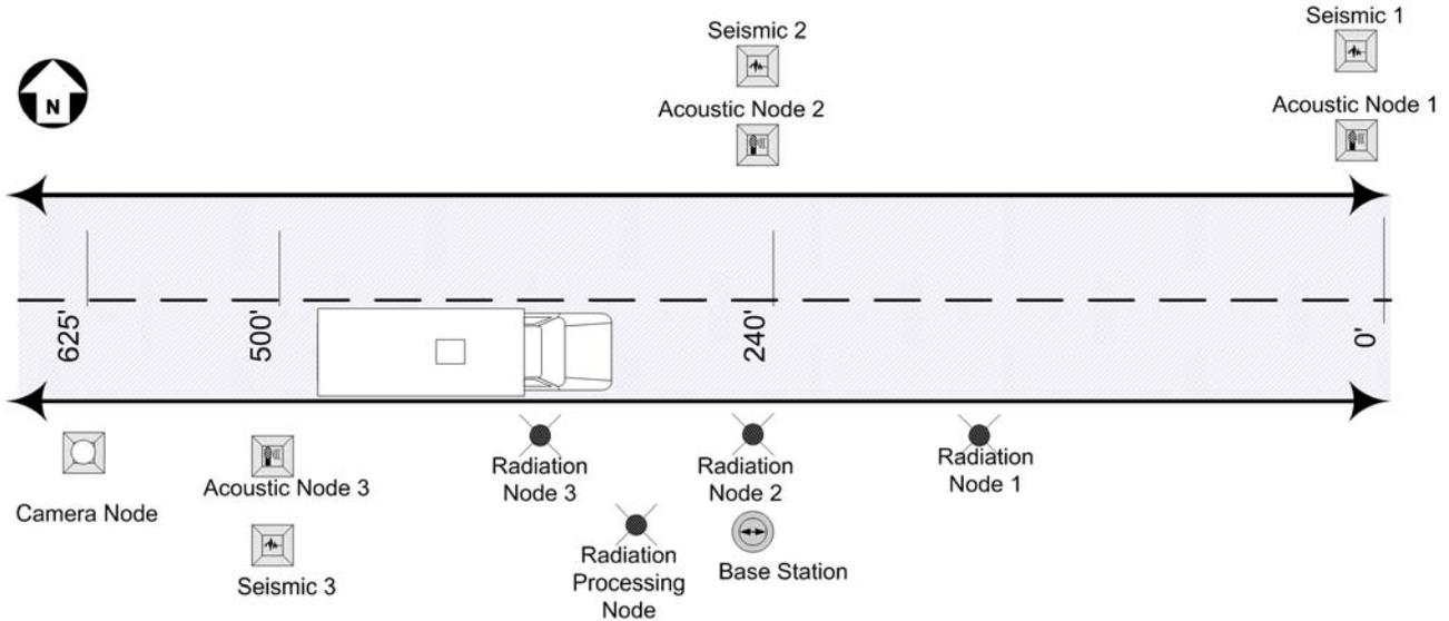
Figure 8 DSN test demonstration configuration
