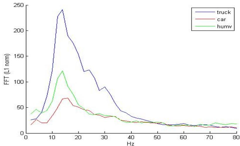
Figure 2 Frequency characteristics of seismic detection
